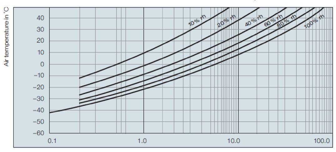
Water content in the air depending on temperature and relative humidity
